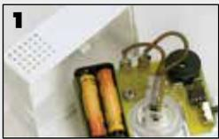
1 Insert the batteries (not supplied) into the case.
